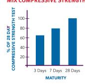
Note: This PROStrength® Extra Strength Concrete Mix compressive strength & Early Strength Development data was achieved under controlled laboratory conditions, at 23 degrees Centigrade. They should be used only as a guide to potential strength as arious factors can impact final strength
