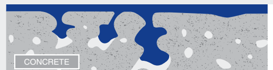
MICROSCOPIC CLOSE UP OF CONCRETE SURFACE USING A SURFACE COATING SEALER
